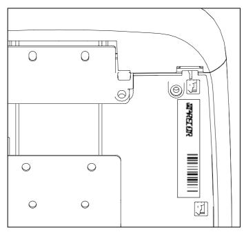
Figure 16: Serial number label location
